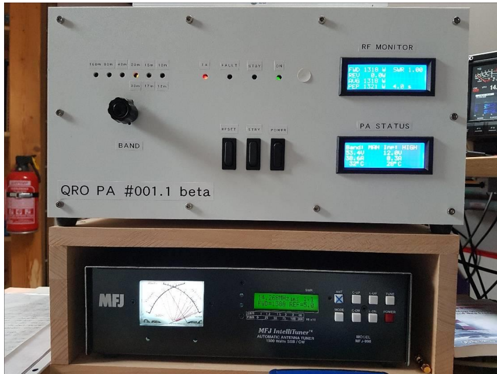
BETA, thermal test 1.3kW+ continuous
